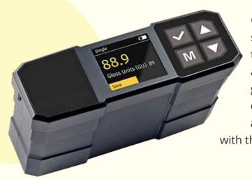
Glossmeter measures Gloss of lacquer and paint surfaces, enamel coatings and other materials in the visible range of spectrum with the aim to assess quantitatively human visual perception of gloss level with the angles of light projection and observation 20°/20°; 45°/45°; 60°/60°; 85°/85° and also diffuse reflection (or brightness) measurement with the angles of illumination and observation 45°/0°.
