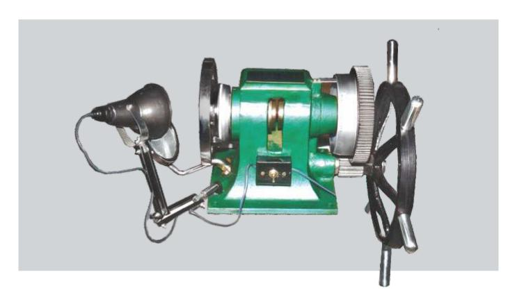
FIE Erichsen Tester is designed to carry out Erichsen Cupping Test on metals. Quick clamping and manual operation facilitates faster and trouble free working of the machine.
